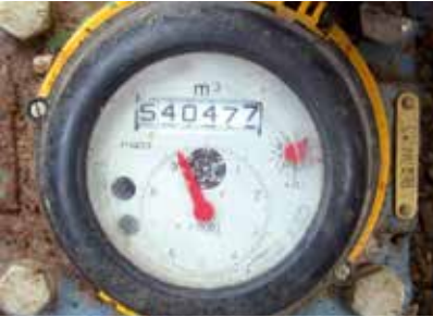
Example 3 - this is 2” meter on a main supply line. It currently reads 540477.92 m³.
