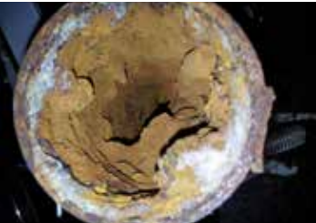
Example of pipe before replacement by PP-R (Polypropylene Random)
