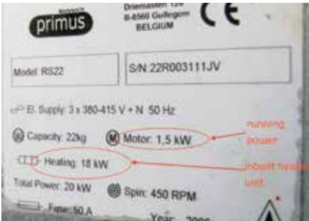
Figure 2 Product specification sticker showing “running power” and “inbuilt heating unit”. These figures should be input in Rows g and h in Worksheet 4, respectively.
