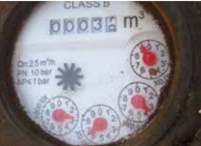
Example 1 - we can see the 8 and know that as it is moving upwards, we have not yet achieved that i.e. the reading is “7”. Looking to the sub-dials below the first one reads 9, the second one 3 and so on. This gives the final reading of 37.9362m³.
