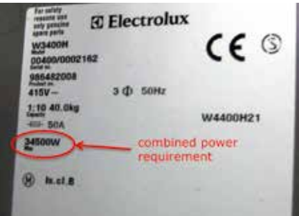
Figure 3 Some machines only detail the total power consumption. In such a situation, you can estimate that 20% of the total power will be required for running power (Row g) and 80% for heating (Row h)
